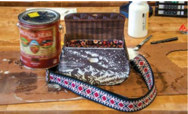
A wooden purse built at Cortez Makerspace by a full-time maker as a birthday gift. The body is laser-cut with a flexible hinge pattern that lets the wood curve, and the fabric lining and interior pockets were sewn in the makerspace as well. The piece is not a contest entry; the maker is entering the Innovation Challenge separately. (Photo by Mercedes Howard / Cortez Makerspace)
