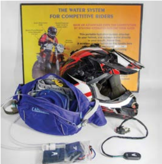
A hands-free hydration system entered in the Cortez Makerspace Innovation Challenge, shown with the maker's explanatory display. Water flows for as long as the rider holds the handlebar button, in a continuous stream or short bursts, with no need to slow down. The system runs on a rechargeable 12-volt battery, and the complete pack weighs about 1 pound, 3 ounces. (Photo by Mercedes Howard / Cortez Makerspace)
